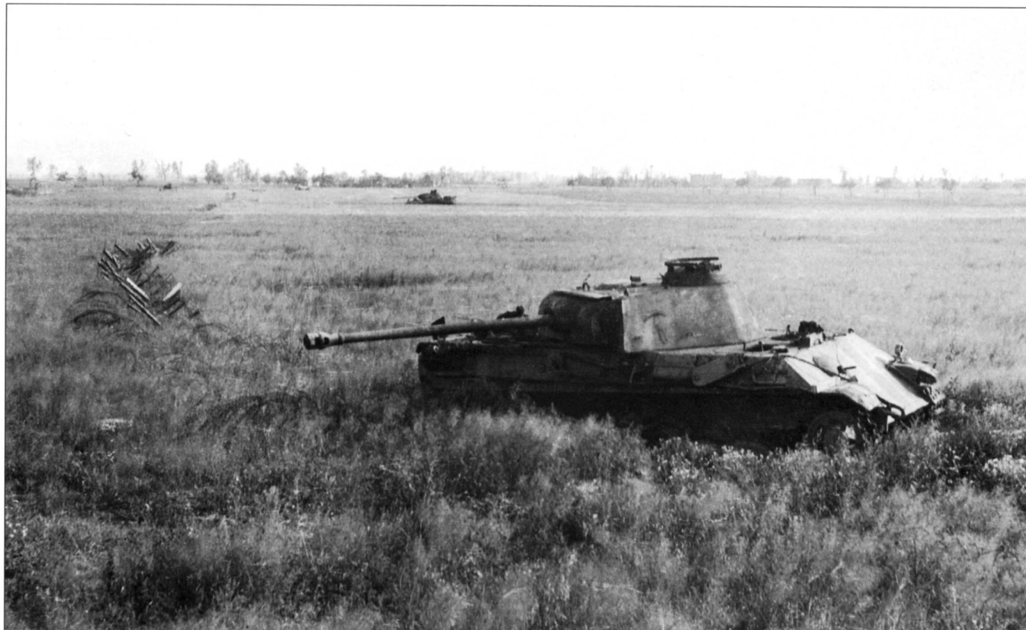
This photograph of the same scene was taken from a different angle. It shows a final series Pz.Kpfw. V Ausf. G Panther with a chin-type gun mantlet used to prevent shells from deflecting onto the thin roof. Note the three-color camouflage pattern seen on the glacis.
