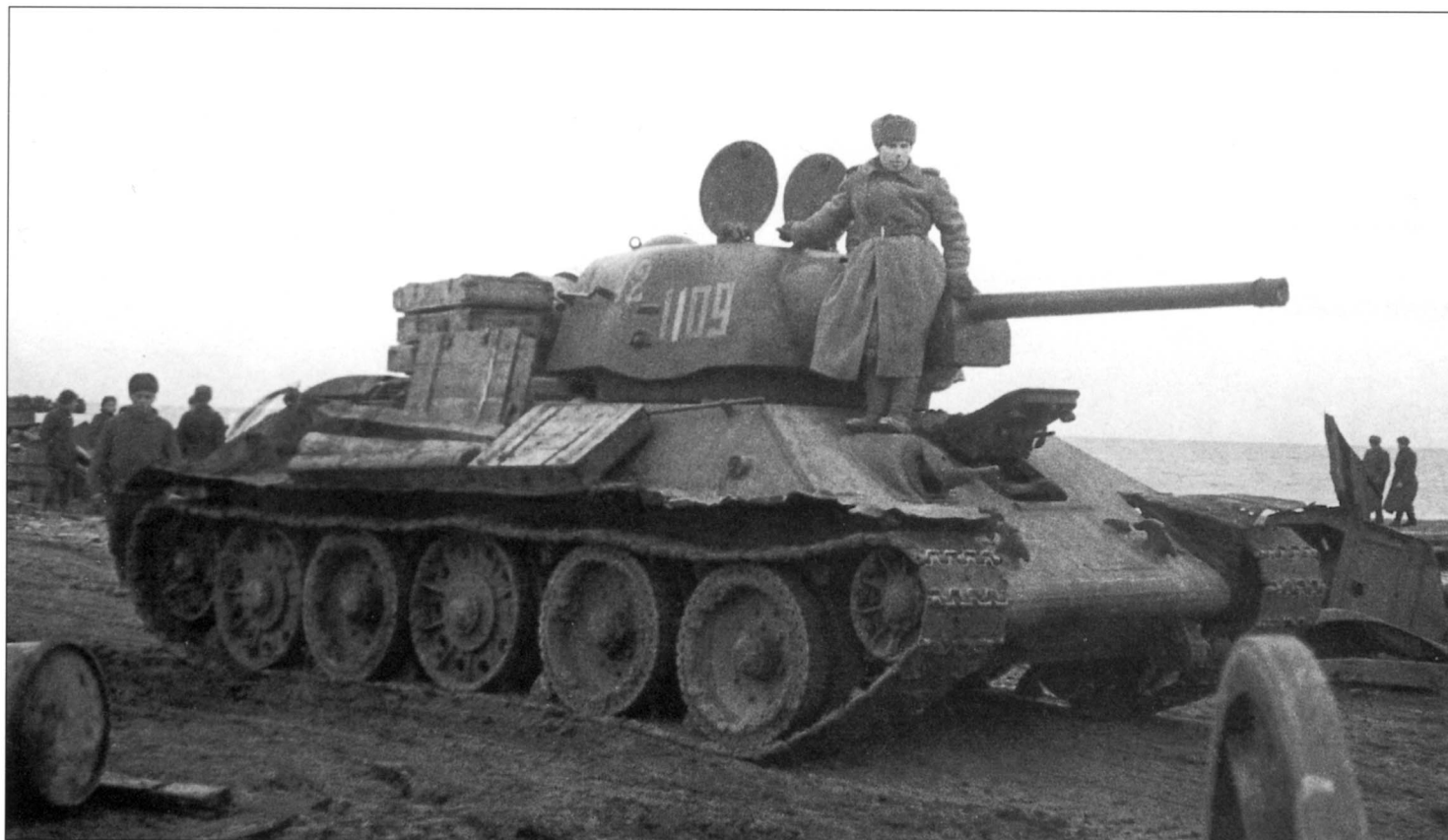
This T-34 Model 1942 with the Uralmash turret typical of the Chelyabinsk Tractor Works factory was photographed in the Crimea in the spring of 1944. The turret is marked with two different numbers: 12 (probably in yellow) and 1109 (in white), and the tank is equipped with a lot of combat equipment — boxes with gun ammunition and a fuel drum behind the turret. Note that the tank has no radio antenna, so it may not be fitted with radio equipment.
