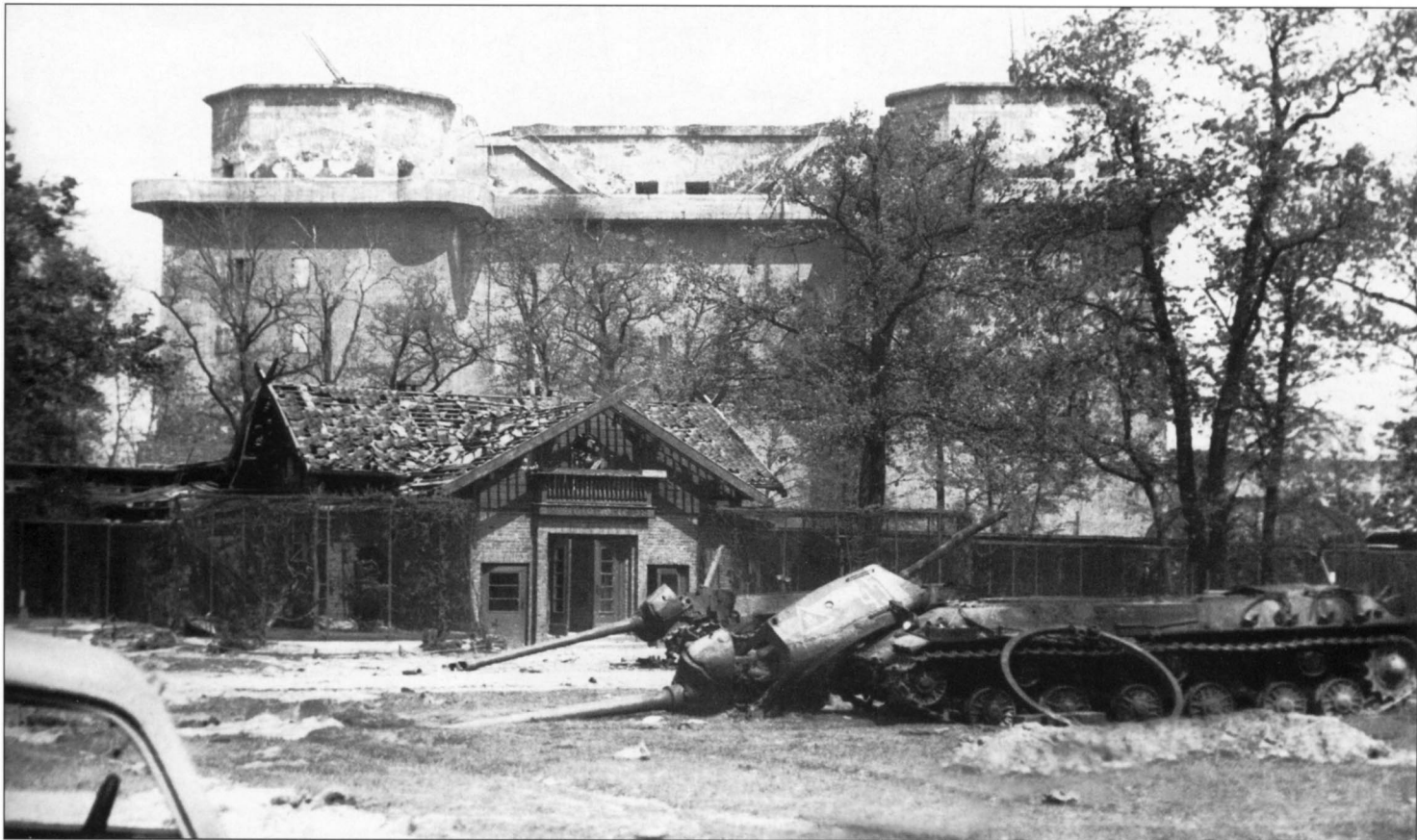
Two IS-2 heavy tanks demolished by German defenders. This photo is a good commentary on the quality of Soviet tank production. Both tanks lost their turrets after receiving hits, and both of them were blown to pieces from explosions or the shock of the collision with the ground. Note the interesting markings on the nearest turret. There is a white band around the turret that is interrupted by unit markings (white triangle with the Russian letter "N"), the number "45" (tactical markings) in white and a vertical band from the white cross painted on the top plate of the turret.
