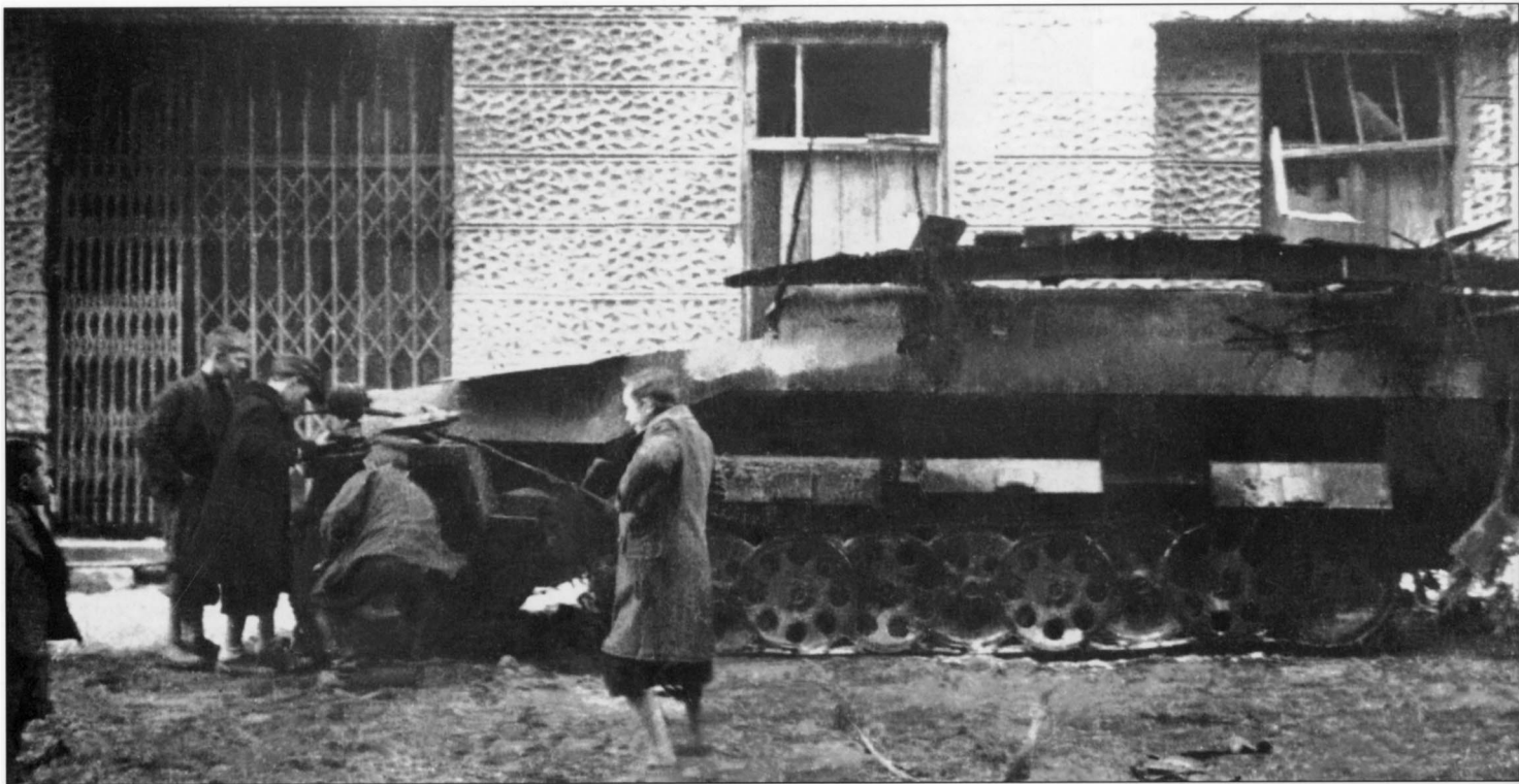
This Sd.Kfz. 251/7 Ausf. D Pionierpanzerwagen was left abandoned on a German street. Note the remains of the standard German camouflage seen in the final period of the war. It was composed of three colors — dark yellow, brown and green, which were painted in equal proportions.
