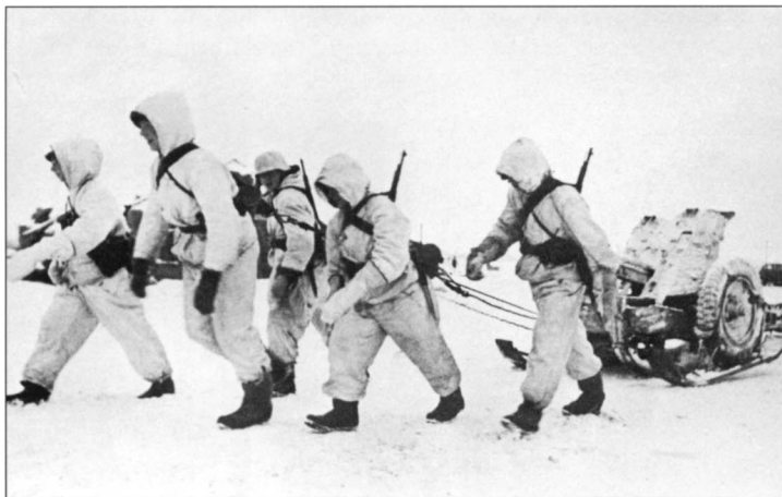
The final stage in the evolution of the Panzerwaffe motorization. Here a 3.7cm PAK 36/37 gun is towed by soldiers during the winter of 1942/43. The specially prepared skis for these guns were quite common among the German units during this winter season.
