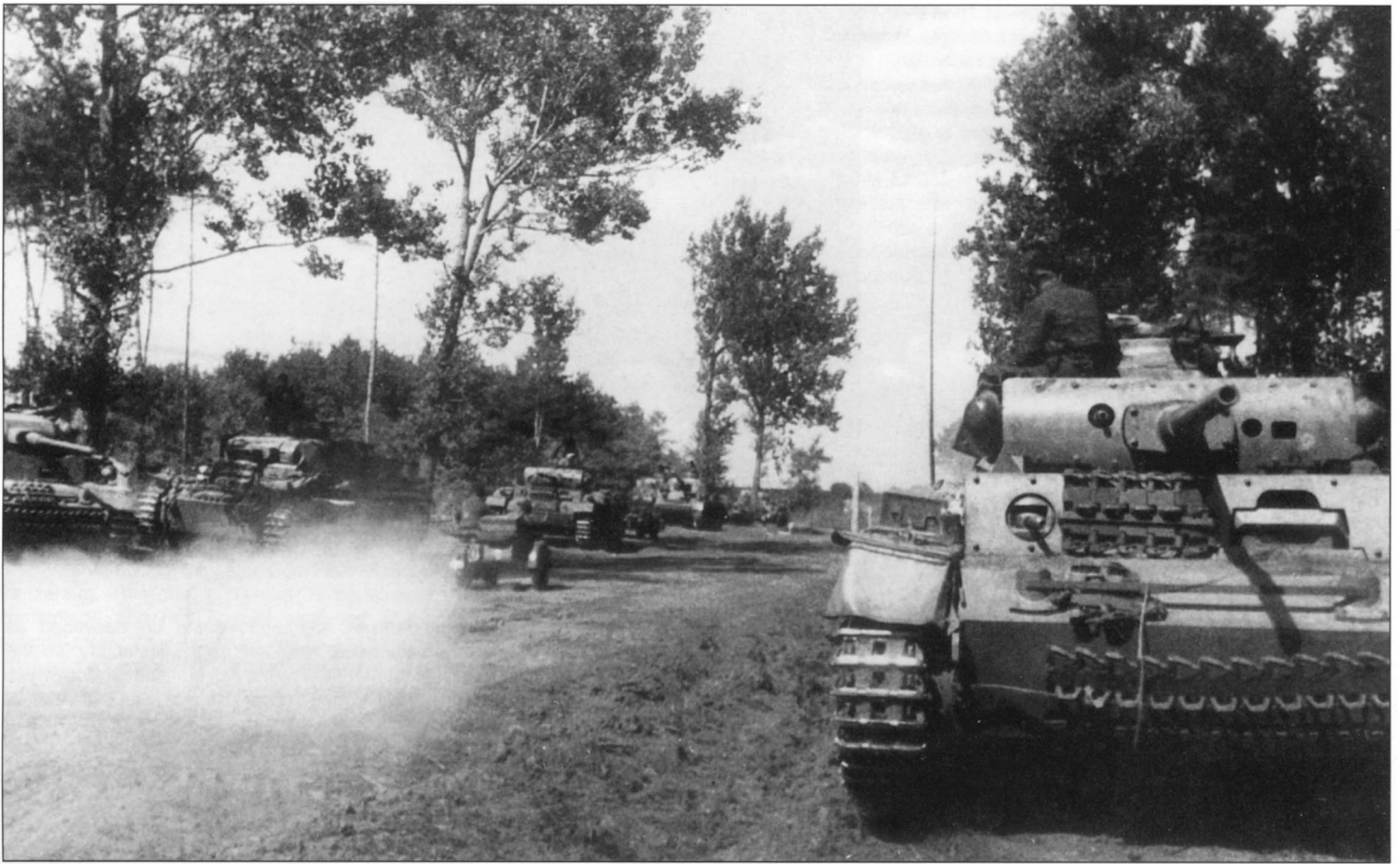
A column of Pz.Kpfw. IIIs from an unidentified division. The tank at the right is the standard version, but the one at the left lacks additional mantlet armor. It also features a very strange, square-shaped hatch in the superstructure frontal plate where the machine gun position should be. Behind this tank is a Pz.Bef.Wg. III Ausf. H fitted with a dummy 3.7cm gun. Note that none of the tanks seen in this photo have side skirts.
