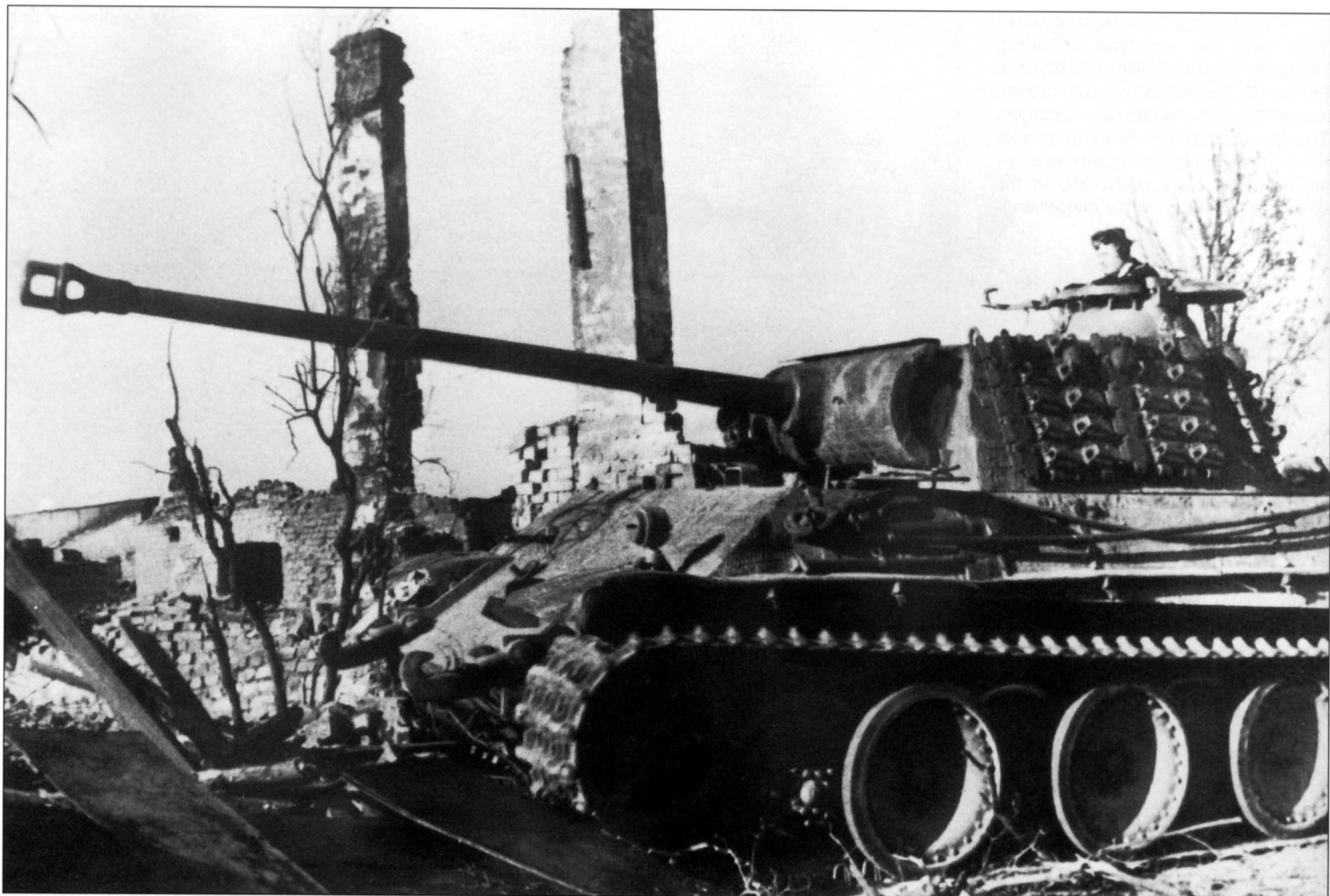
A Pz.Kpfw. V Ausf. G in action in a destroyed village. This vehicle is from the early series, without reinforced armor on the mantlet below the gun. The towing hooks are fixed in working position. Note that the black national cross at the very front on the side of the superstructure appears to be composed of just a couple of brush strokes. There are no other markings. The anti-tank rounds fired from a Panther tank could penetrate armor plating of about 150mm at a 30 degree angle at 1,000 meters, so its ballistic capabilities were much better than Soviet 85mm guns on the T-34 or SU-85 vehicles, and very similar to those of the IS-2's gun.
