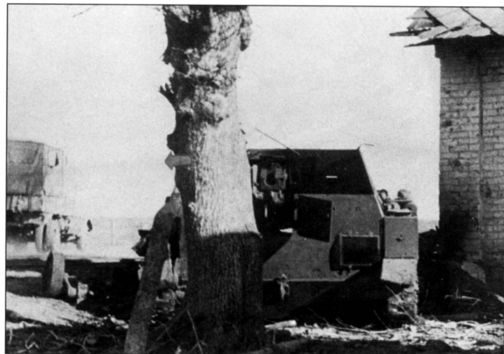
German rounds struck this SU-76M on the outskirts of a village. Note the dark color of the vehicle's interior. It was painted with a dark green camouflage paint, but in 1944 the Soviets introduced white interiors to all their armored fighting vehicles.
