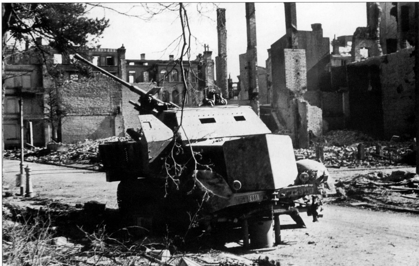
Wreckage of the Panzerwaffe found by victorious Polish and Soviet units in captured Kolberg (Kolobrzeg) in March 1945. This photo shows the remains of a Sd.Kfz. 7/2 armed with a 3.7cm Flak 36 anti-aircraft gun and equipped with an armored cab. Like many of the Panzerwaffe's other wheeled or half-tracked vehicles, this half-track had its wheels plundered for the benefit of a needy Soviet vehicle that suffered from the general lack of spare wheels. The Sd.Kfz. 7/2, license plate number "WH-152661", is painted in a three-tone camouflage (small green and brown spots on a dark yellow background).
