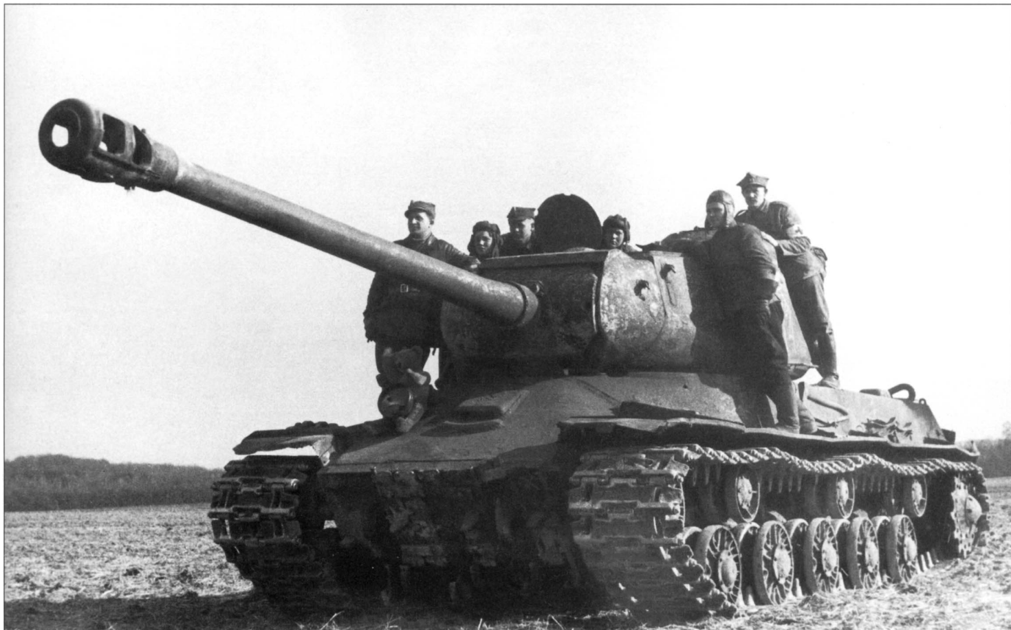
This is an excellent portrait of an IS-2 heavy tank from the Polish 4th SPCzC. It is the later model with a rebuilt frontal part of the superstructure. Note the many details on this tank, including the crew's mascot (a teddy bear) seated behind the front light. The lack of the rear road wheel was quite a common sight in units equipped with these tanks. The Soviets did not care for spare wheels, and when the chassis was damaged by a mine, they simply replaced the damaged road wheel with one from the rear. Remnants of white paint, which was removed soon after December 1944, may be seen on the turret and gun barrel. The clothes worn by the soldiers show just how warm this winter was. This photo was taken in the first half of February 1945!
