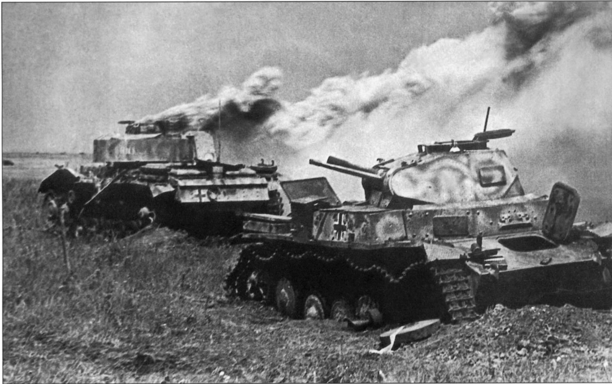
The Panzerwaffe left behind many tanks on the killing fields of Kursk. Here are two of them, a Pz.Kpfw. III (left) and a Pz.Kpfw. II (right). Both vehicles are from a staff unit, as indicated by the tactical number "R10" on the turret skirt of the Pz.Kpfw. III. The interesting camouflage pattern on the Pz.Kpfw. II is composed of dark yellow irregular patterns on a dark gray background.
