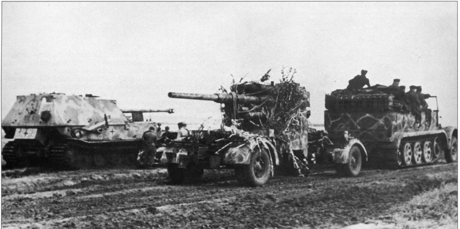
Both the 12-ton Sd.Kfz. 8 half-track (at right) and the 8.8cm Flak 36 it is towing are camouflaged with a dark yellow pattern over dark gray. They are passing by the weapon that turned out to be the hit of the summer of 1943 — the Elephant. During the fighting on the Kursk bulge, the Elephant won immortal fame as the heaviest AFV of this period. In the following decades this vehicle was described almost solely as unsuccessful and basically inefficient in combat. This description is based mainly on one statistic — the number of Elephants that were lost, which was 39 pieces. The losses were, in fact, heavy, but they were only about 50% of the strength of Jagdpanzer Regiment 656 (comprising Pz.Jäg.Abt.653 and Pz.Jäg.Abt.654). It should be noted that the same percentage of losses was experienced in some Tiger units. The German Elephant crews forced the Soviets to pay a very high price for their victories. As of 27 July 1943, during only 22 days of battle, the Elephants destroyed 502 tanks and many other weapons. The camouflage of the Elephant seen in this photo consists of large green spots on a dark yellow background. Note that there is no tactical number.
