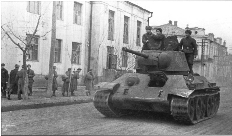
A T-34 Model 1942 passes through a city as it advances toward the Dnieper river in September 1943. Note the markings on the turret and the different width of the road wheels: the first and the last are pierced rubber-rimmed, the second and fourth are the standard rubber-rimmed style, while the road wheel in the middle is the all-steel version.
