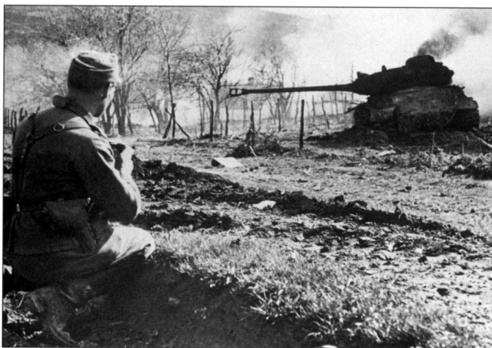
A Pz.Kpfw. V Ausf. G in action in a destroyed village. This vehicle is from the early series, without reinforced armor on the mantlet below the gun. The towing hooks are fixed in working position. Note that the black national cross at the very front on the side of the superstructure appears to be composed of just a couple of brush strokes. There are no other markings. The anti-tank rounds fired from a Panther tank could penetrate armor plating of about 150mm at a 30 degree angle at 1,000 meters, so its ballistic capabilities were much better than Soviet 85mm guns on the T-34 or SU-85 vehicles, and very similar to those of the IS-2's gun.
