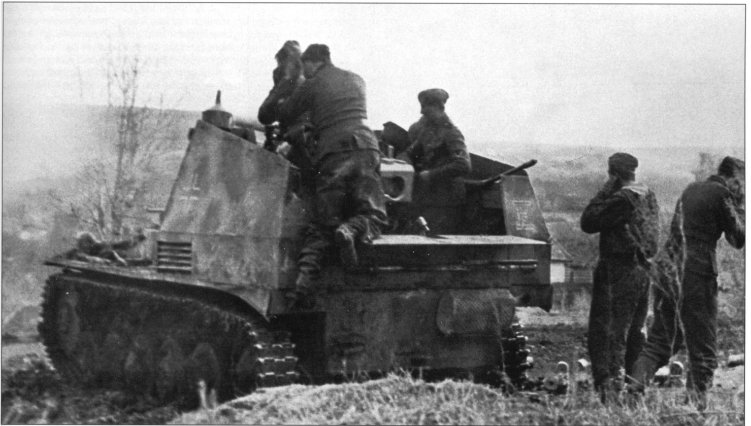
Crew members of a light self-propelled howitzer protect their ears from noise as their gun goes to work. The Wespe was the only vehicle of the Panzerwaffe in which the 10.5cm howitzers were installed. The conception of this vehicle was the same as all the other self-propelled guns of the Panzerwaffe. An obsolete tank chassis was adapted for the leFH 18 howitzer, so the Wespe gun crew had little space for comfortable work. Therefore, only two soldiers were stationed in the combat compartment, while three others, as well as the ammunition, remained outside of it. This Wespe is camouflaged with green or brown spots and marked with the letter "E", which indicates that it is from an independent artillery unit used by the staff of an army corps.
