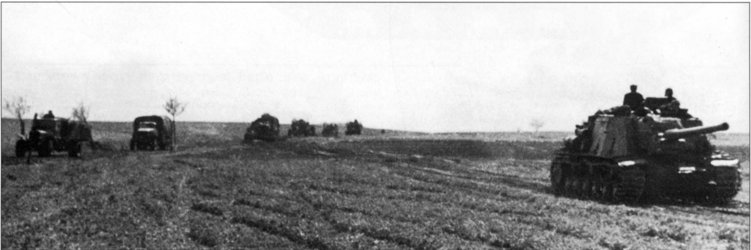
An ISU-122 heavy self-propelled gun and a column of trucks (in the background) are shown on the march toward an assembly area. The ISU-122, designed just after the ISU-152, was a powerful vehicle armed with a 122mm A-19 gun, but it was also slow, not maneuverable and had a short range. Like the ISU-152 it was very similar to the German Elephant, so it had to be used properly and thoughtfully if success was to be achieved. However, the actual performance of the ISU-152 on the Ukrainian battlefields in the winter of 1944 was a disaster: two regiments of these vehicles were wiped out in one action. These losses were so heavy that a special commission had to visit the front to find out the reason for this collapse.
