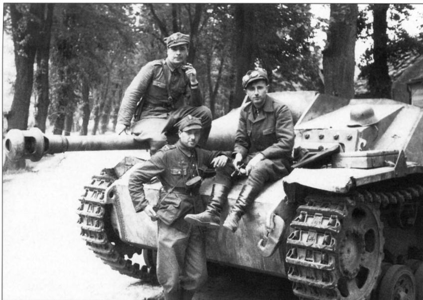
During the pursuit action across the Pomeranian fields in the first week of March 1945, Polish troops captured 22 tanks and self-propelled guns. Among them was this StuG III Ausf. G, which was captured by the Polish 4th Infantry Division. Note the steel return roller that replaced the standard one in late 1944.
