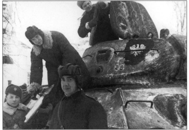
A close-up of a T-34 Model 1942 from the Polish 1st Polk Czolgow photographed during the loading of ammunition during the winter season. Note the many details of the construction of the tank produced by Factory No. 112, such as the raised casting of the number “26” on the side of the turret, which may indicate the production series. This white residue on the armor is the remains of the removable white paint used for winter camouflage. The white eagle, the national insignia of the Polish People’s Army, was painted with the help of a stencil in a dark color (maybe black) over the tank’s base color. The shells passing through the hands of the crew are high explosive rounds.
