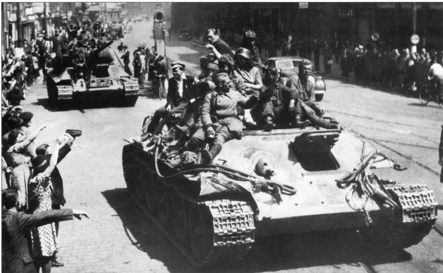
A T-34 recovery tank travels down a street in Prague during a victory parade in May 1945 just after the liberation of the city. The T-34 recovery tank was built in front-line workshops utilizing damaged tanks with turrets that were beyond repair. The 1st Ukrainian Front under Marshal Ivan Konev was the main force assigned the task of liberating Prague. Feldmarschall Ferdinand Schoerner, who was defending Prague, finally surrendered on 11 May.
