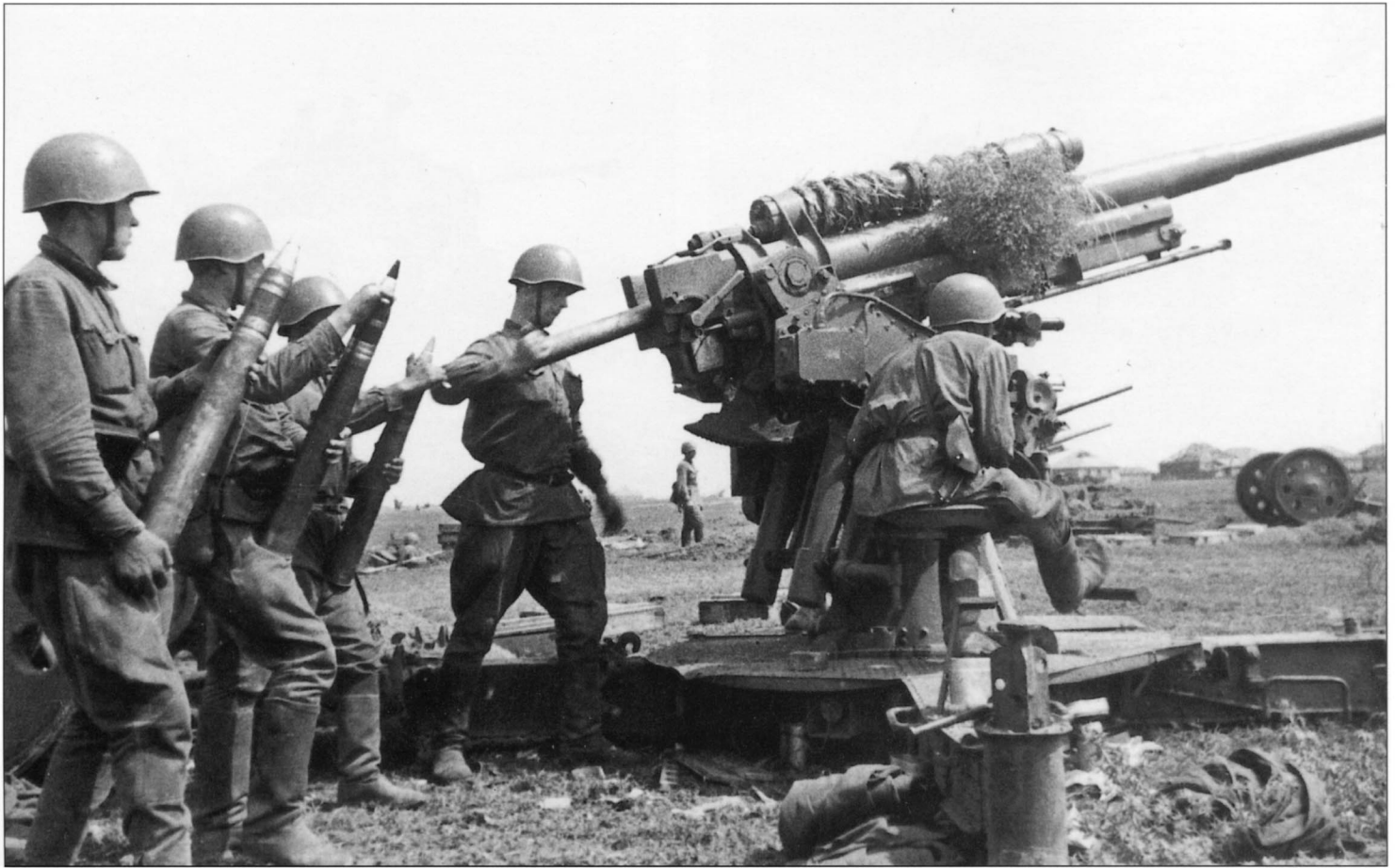
The crew members of a Soviet 85mm Model 39 anti-tank gun get ready for action. This gun was almost the equivalent of the German "88", being just a bit less powerful. An anti-tank round from this gun could penetrate 100mm vertical armored plate at a range of 1,000 meters (about 1,100 yards), while the "88" could penetrate almost 140mm of armor at a 30 degree angle.
