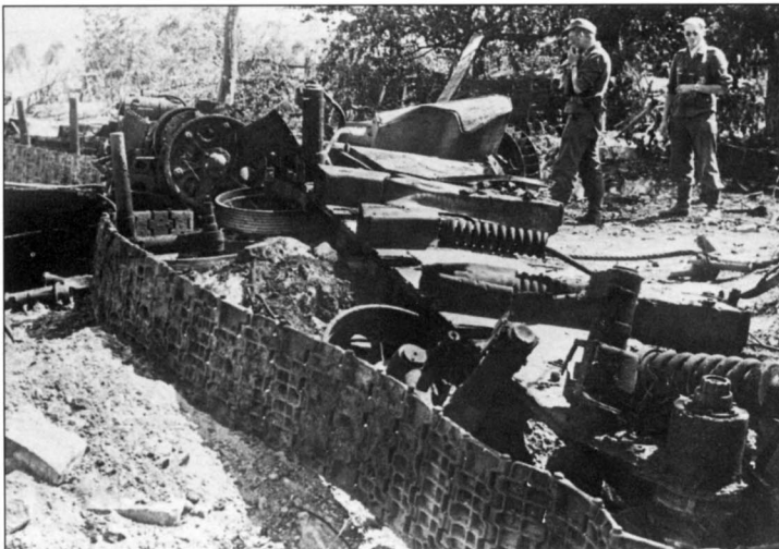
What we see in this photo are the few remains of a T-34 that exploded after receiving a direct hit from an 8.8cm round. The armor-piercing rounds of 8.8cm KwK36 L/56 and 7.5cm KwK42 L/70 guns had tremendous power and easily penetrated the low-quality steel armor of the Soviet tanks produced in 1942 and early 1943.
