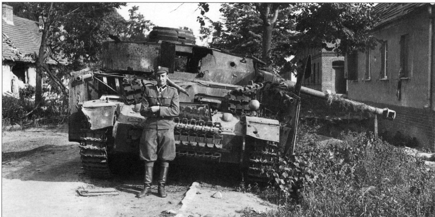
Another German vehicle abandoned on a Pomeranian road — a Pz.Kpfw. IV Ausf. J with wire mesh side skirts and standard armored skirting on the turret. Note the additional armored plate bolted onto the frontal wall of the superstructure and the two entry holes where rounds hit the turret. One of them blew off the doors and a piece of turret in the area at the upper right corner of the hatch.
