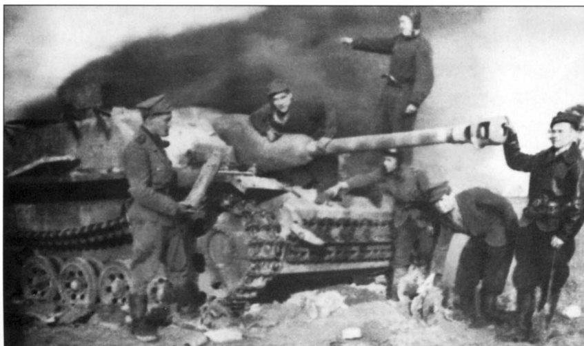
Another German vehicle abandoned on a Pomeranian road — a Pz.Kpfw. IV Ausf. J with wire mesh side skirts and standard armored skirting on the turret. Note the additional armored plate bolted onto the frontal wall of the superstructure and the two entry holes where rounds hit the turret. One of them blew off the doors and a piece of turret in the area at the upper right corner of the hatch.
