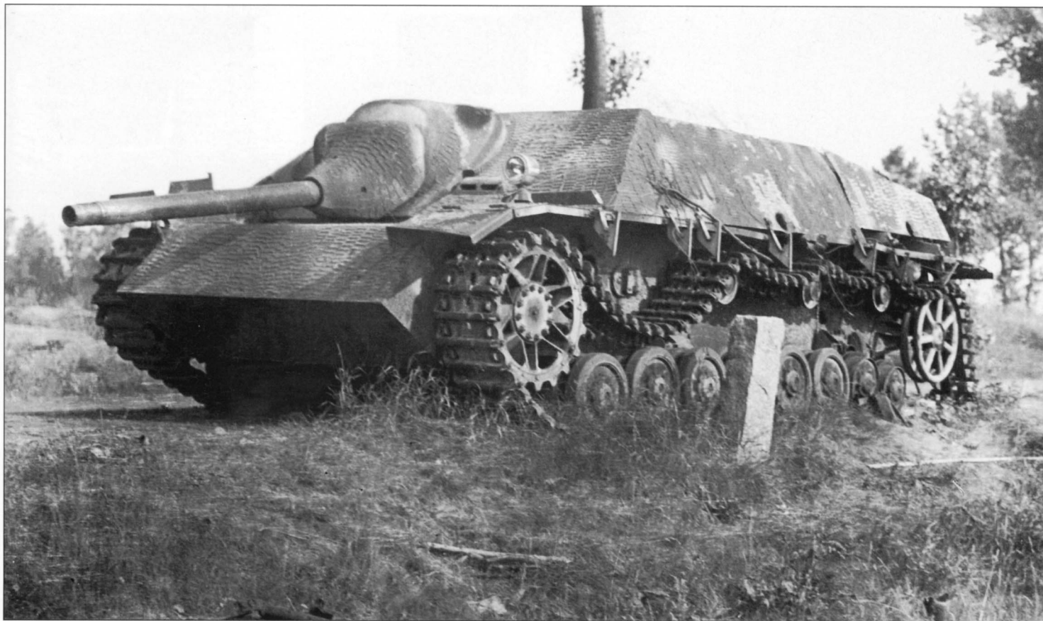
A Jagdpanzer IV with a 7.5cm gun (minus its muzzle break) that was knocked out in the Dresden area. This self-propelled gun received no fewer than three hits in the left side — one in the superstructure, another in the engine compartment and the third in the hull near the middle return roller. Note the tactical number "300" painted on the front part of the side plate. The vehicle has a coating of Zimmerit anti-mine paste on its armor, but it has lost its side skirts.
