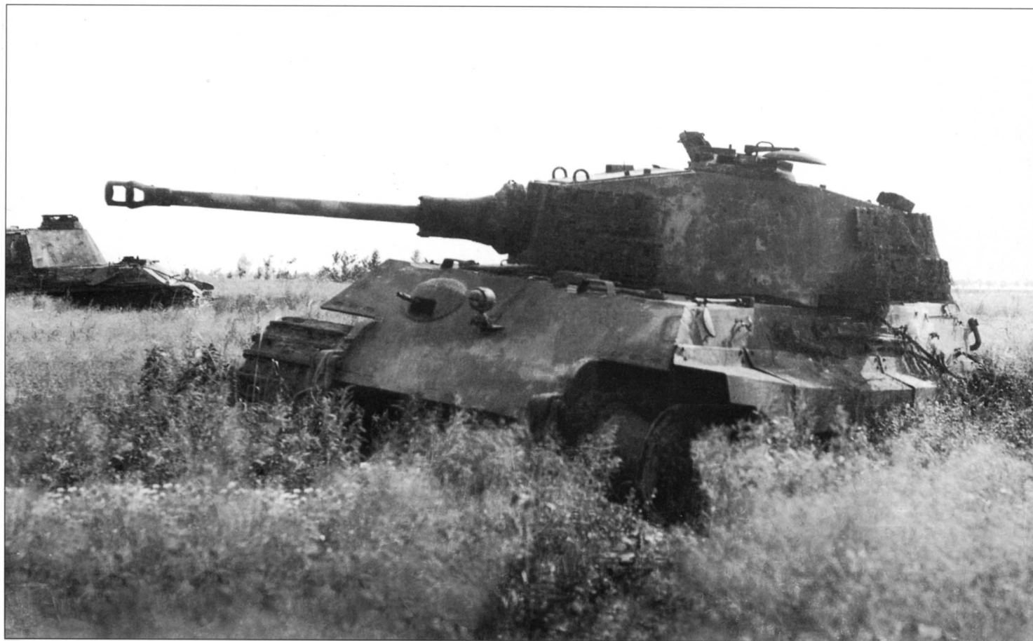
And here is a small surprise — a Pz.Kpfw. VI Ausf. B armed with the 7.5cm KwK42 L/70 from a Panther tank. The standard model of Tiger II was armed with the 8.8cm KwK43 L/71 gun. The reason for rearming this tank is not known. However, it is possible that the original gun was damaged and then replaced with the only one available at the time. This tank was probably from sSS-Pz.Abt.502, which was assigned to defend Berlin.
