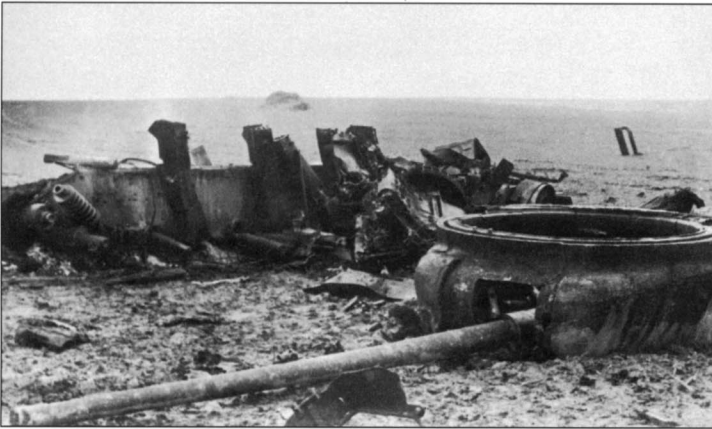
The remains of a Soviet KV-85 heavy tank destroyed somewhere on the flat landscape of western Ukraine. This was one of the rarest series of Soviet tanks. Nevertheless, one of them was captured by the Germans and tested at the Kumersdorf testing ground. There is no doubt that the tank was hit hard at short range by an 8.8cm anti-tank round, or maybe even by a Panzerfaust warhead, which caused the internal explosion of the ammunition.
