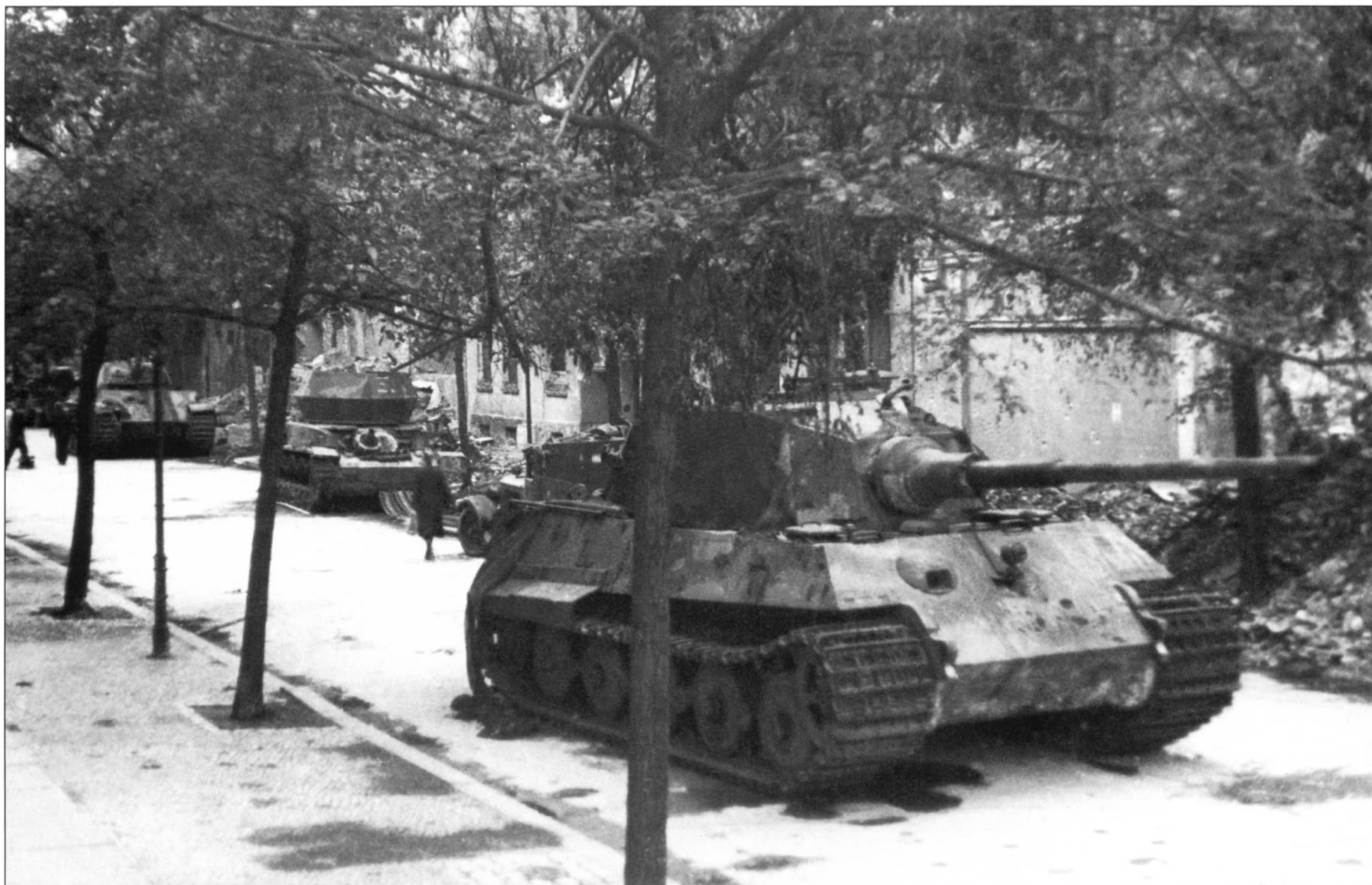
Another Tiger II (in the foreground) abandoned on a street in an unknown German city somewhere in the Berlin area. Note that the tank's muzzle break and machine gun are missing. Behind the Tiger II is a Flakpanzer "Wirbelwind" and a Panther.
